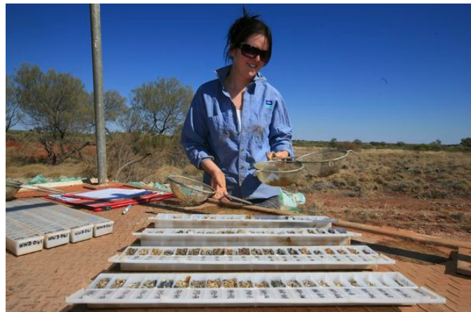
Drill chip sampling: hole WWS041 returned an intersection of 12 metres of anomalous Manganese grades.
